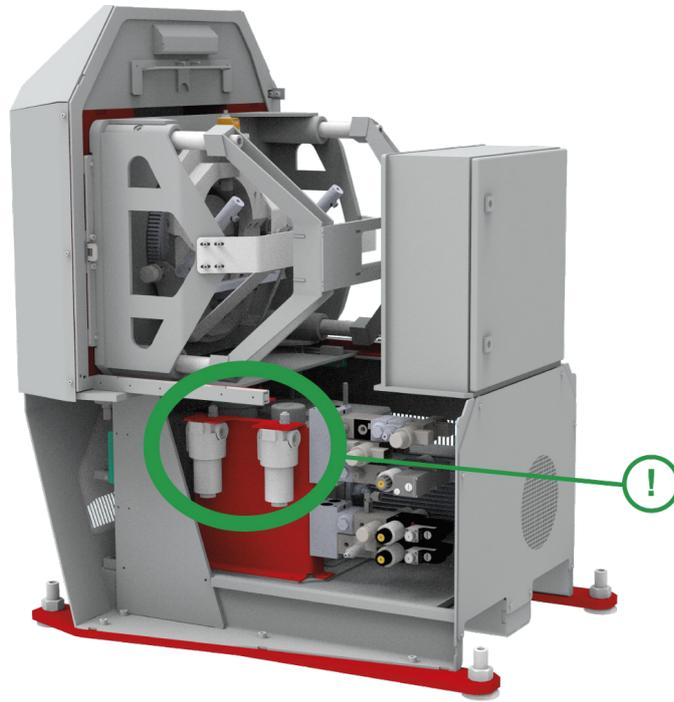
*! Hydraulic unit filters with indicator on top*
