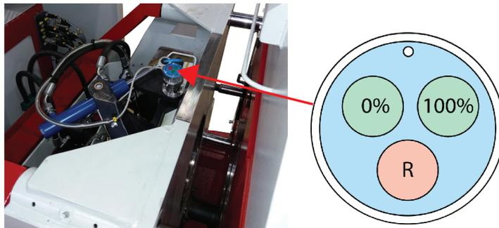
All angle adjustment plates have to be removed before starting to make settings of the angle sensor (Angular Position Transducer). The setting is not accurate with adjustment plates!
