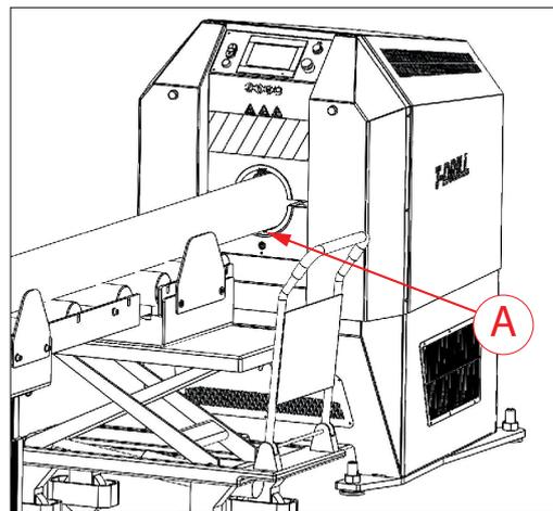
➔ **NOTE!** The pipe must be lowered to the roller track in a controlled manner to avoid damaging the track. A falling track will cause a high risk of injury!
