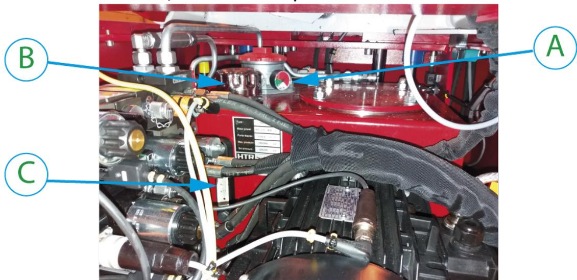
*Hydraulic oil container (pictured from behind the machine): A. Oil pressure gauge, B. Oil refill cap, C. Oil temperature / amount gauge*
