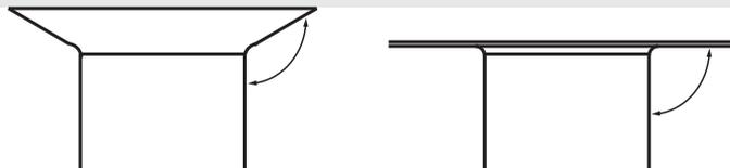
The angle of the flange to be made is adjusted by putting chosen angle adjustment pieces to the flanging unit forming pin frame. Tube material has great influence to the flange forming, and the correct piece size can only be found through testing.
