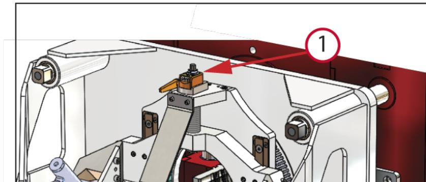
1. Pin height adjustment scale screw
