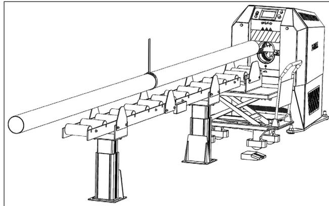
Lift the roller track a little higher than the pipe clamp lower surface. (A = 5-25 mm).
