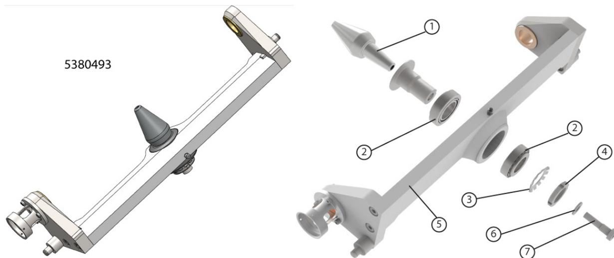
*Swinging arm assembly 5380493: 1. Forming pin, 2. Bearing, 3. Spring washer, 4. Lock nut, 5. Swinging arm, 6. Washer, 7. Fastening screw of the pin (M10 socket head cap screw, 8mm key)*
