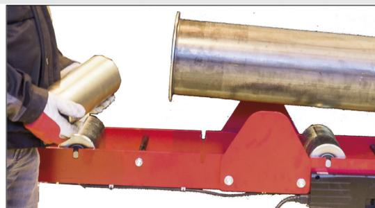
The roller track can handle pipes  $\varnothing$  20 mm ...  $\varnothing$  219,1 mm.
