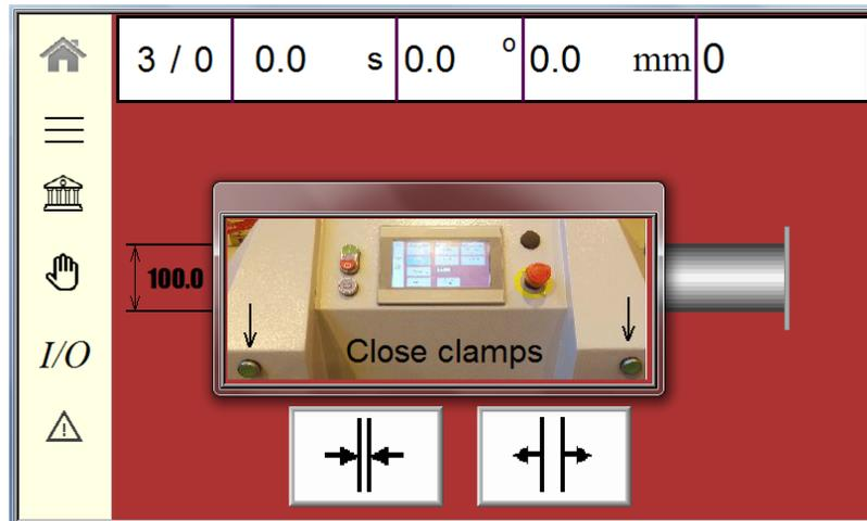
*If the clamp is not completely closed, there will appear a pop-up advising to close the clamps when trying to start work cycle (push work cycle button).*
