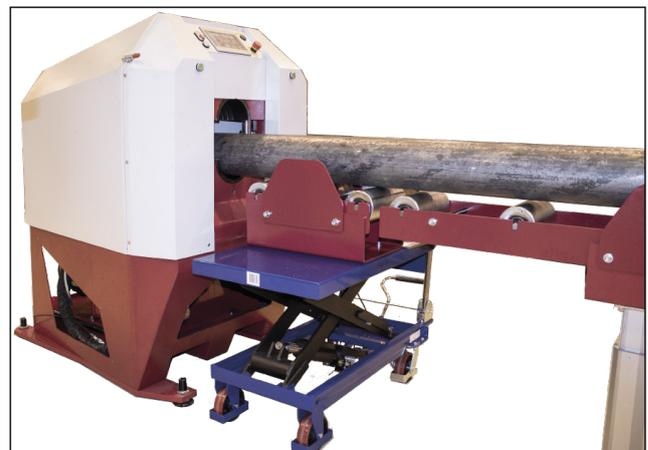
➔ **NOTE! Always lock the wheels of the lifting trolley before moving the pipe to the roller track!**
