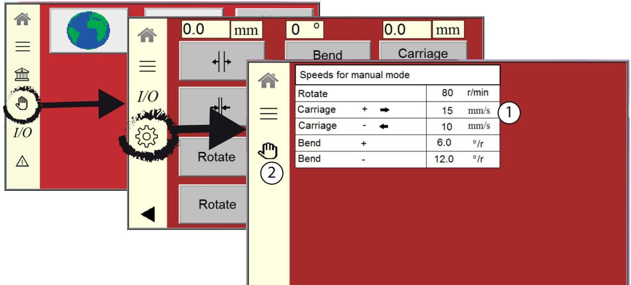
1. Tap setting value field to open keypad; set desired speeds for manual drive. (Note: Machine has factory preset values and factory set limitations for speed values!)
