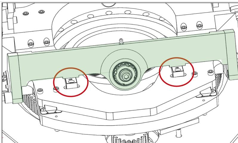
The angle of the flange is mechanically limited with the adjustment plates as the swinging arm leans to the plates, and also an electric limit switch controls the flanging program. It is important to add the angle adjustment piece value to the program settings!
