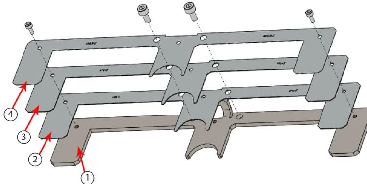
Backstop plates: 1 Base plate, 2. 1st backstop, 3. 2nd backstop, 4. 3 rd backstop
