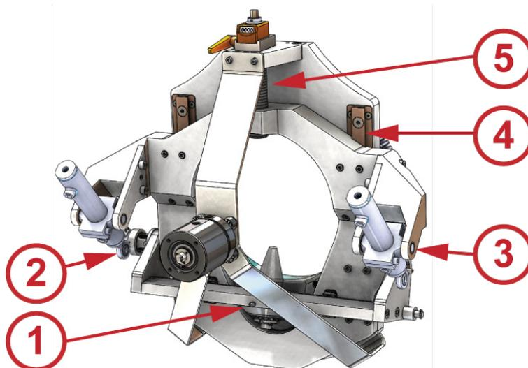
1. Lubricate the forming pin through the grease nipple with grease gun, 2. Check joints for wear and tear occasionally, 3. Check bearings for wear occasionally, 4. Wipe slides clean, lubricate with spray grease, 5. Wipe thread clean occasionally, lubricate with spray grease.
