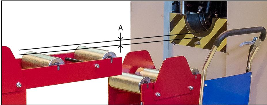
Lift the pipe with a crane to the roller track, use a lifting strap.
