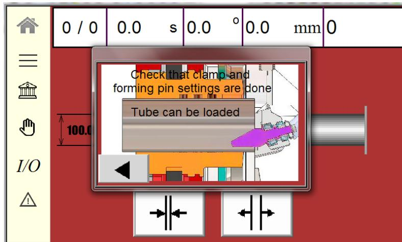
First run of a new program: When a new program has been loaded from the library, the machine will ask to check the clamp and forming pin settings. When the carriage is in the starting position, a pop-up will appear to inform that the machine is ready and tube can be put into the machine.
