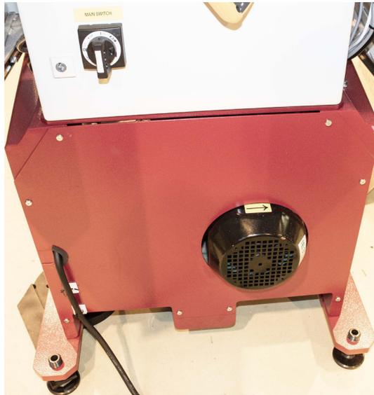
2. Check the rotation direction of the motor, correct direction is marked on top of the motor.
