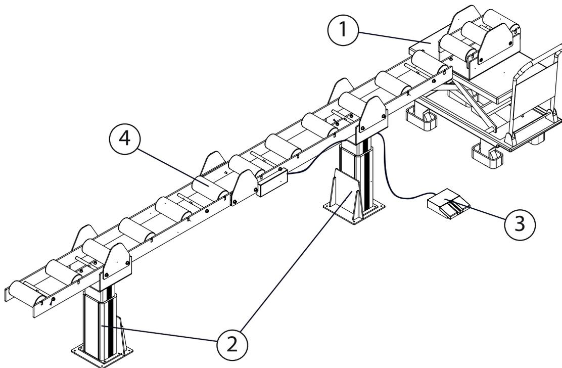
Parts of the roller track: 1. Lift trolley, 2. Roller track lifting device, 3. Roller track operating pedal, 4. Support roll
