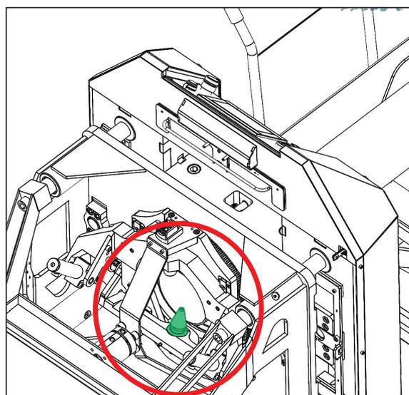
➔ **NOTE!** Do not push the pipe in to the machine too hard, the heavy pipe may damage the forming pin.
