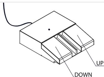
The track operating pedal is marked with stickers, which is the up, and which is the down movement of the roller track. A hand control is also available.
