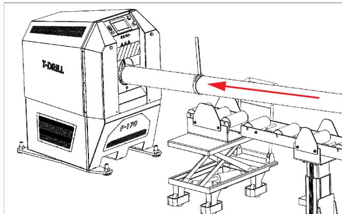
**➡ NOTE! The pipe must be lowered to the roller track in a controlled manner to avoid damaging the track. A falling track will cause a high risk of injury!**
