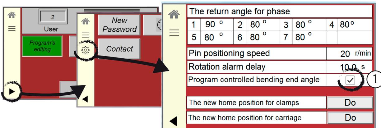
USER2 screen, tap “gear”-button and tap to check and activate “Program controlled bending end angle” function in flanging program: Set bending end angle when making the program. (Without setting, the bending end angle is 90°)
