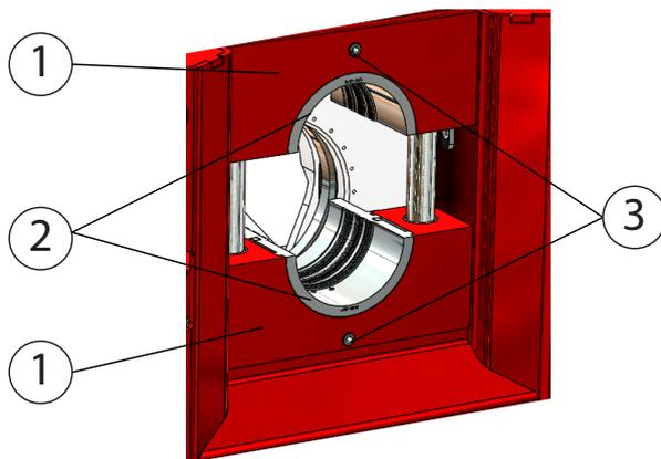
*1. Clamping device jaws, 2. Clamps, 3. Clamp locking pins.*
