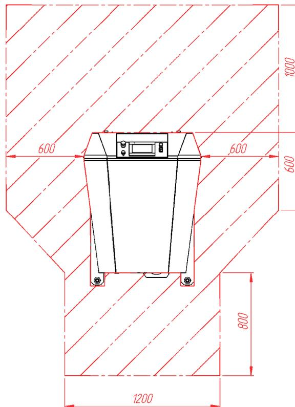
*Machine measures and required working space*
