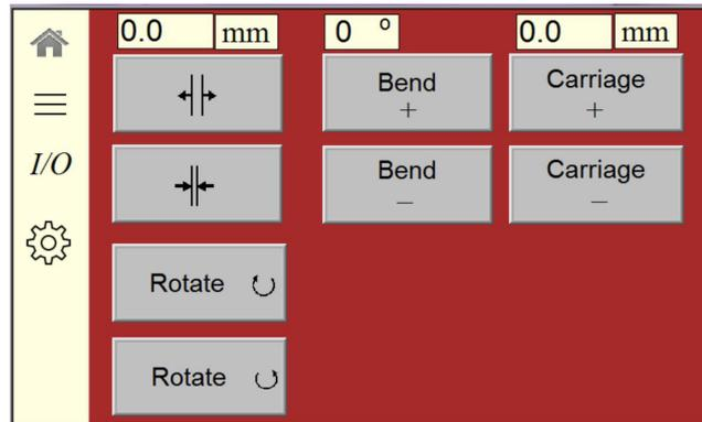
The machine is controlled manually from the control panel. The machine cover must be closed to perform any movements.
